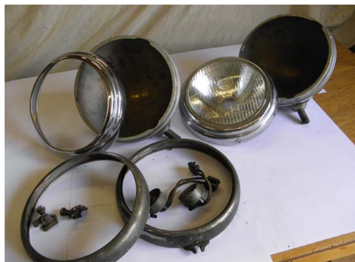
Pair of Lucas LB140, same as L140 but have the adaptor rims to take 7" light units – both rims included but only one light unit but standard rims included to convert to standard L140. Reflectors and glasses needed to finish. £150.
