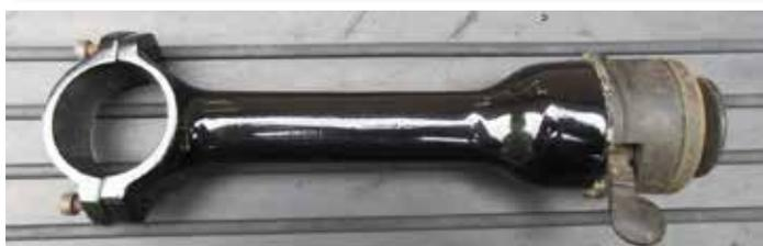
The picture shows the back of the new stalk with the cable entry point. A minimum order of 10 is required and the castings will come as in the picture so will need cutting, drilling, tapping, filing and smoothing. The price would be £50. The 'standard' triple M horn/dip switch can be adapted to fit or the T Type one. Let me know in the first instance if you would be interested.
