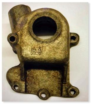
This is the end plate, speedo drive holder, from a 3 speed D Type gearbox which is interchangeable with that on an M Type. Not quite 'hen's teeth' but nearly. Whole D Gearbox very considered too!
